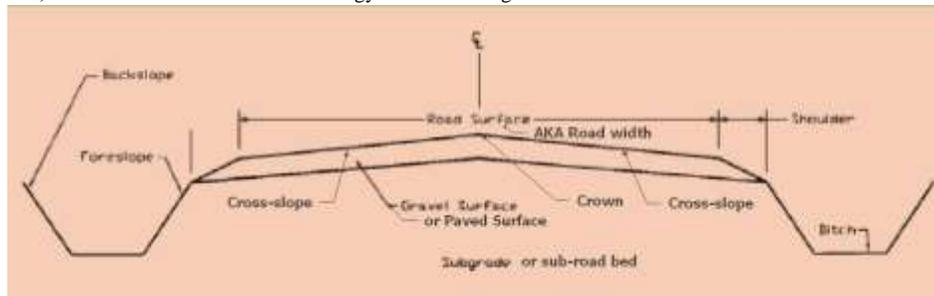
Figure 2- Roadway section features
